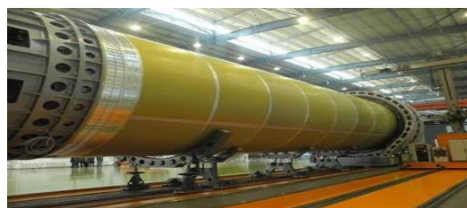
Fig. 4 5 m diameter lightweight cryogenic tank
